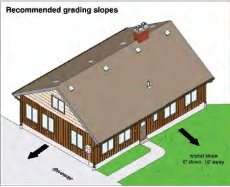
Illustration Grading Slope
